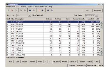
The Production Runs screen gives a birds-eye view of the production for a given day. This screen is updated as pieces are ordered, produced and loaded. Details for each run are available at the push of a button, including the status of individual orders and pieces.
