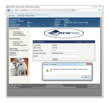
Validation prompts can be added to each operation to require scanning of FR lot numbers, subassemblies, or special components. No operation is allowed to complete until all required fields are entered.
