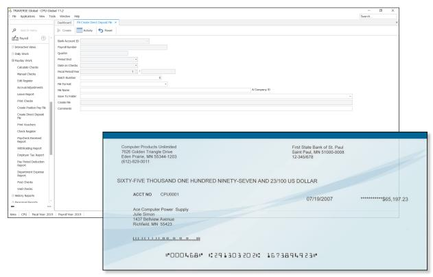
The MICR line on a check allows the check information to be automatically read for quicker processing.
